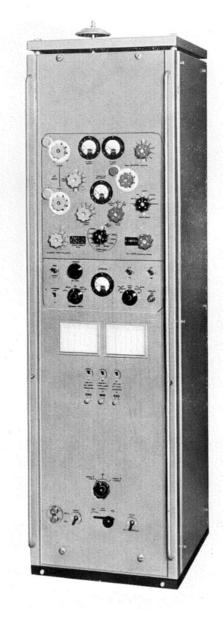
band-pass filter so arranged that its response combines with that of the final stage MF grid circuit to maintain a reasonably constant input level to the final amplifier stage. An isolator precedes the final stage which employs three valves connected in parallel, special care being taken to avoid any parasitic oscillations.
