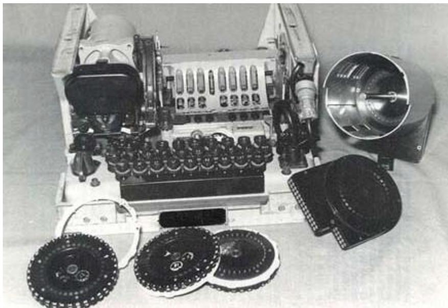
*The KL-7 Electro-Mechanical Cypher Machine used by the New Zealand services.*
