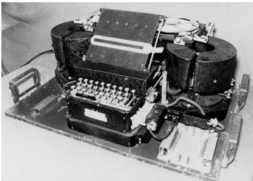
*TYPEX Mark 22 (BID/08/2) fitted with the crossover device for extra security*
