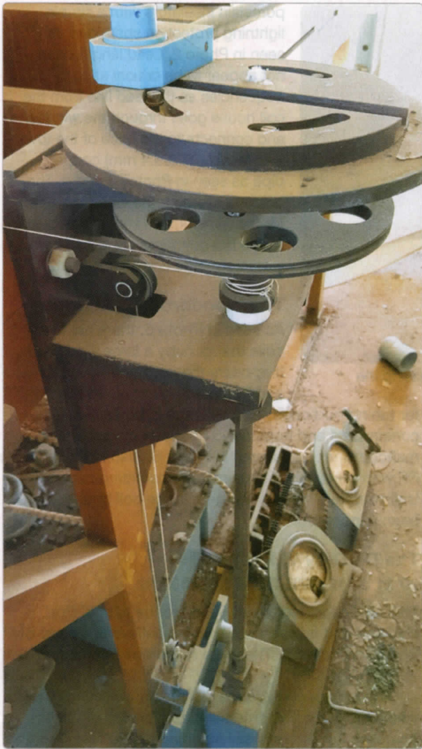
Photo 6: Part of the Woodbrook Coil House tuning mechanism on the side of the coil mounting rack.
