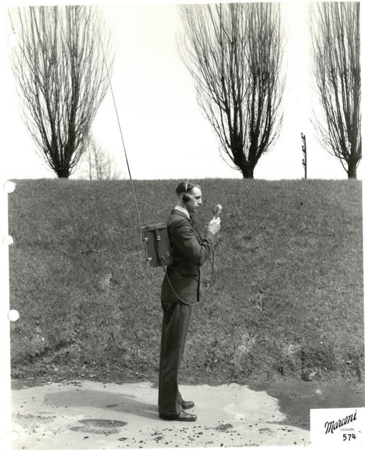
Marconi medium frequency portable transmitter-receiver for broadcast pick-up, 3 watts output, type CBl. (strapped on man's back).
