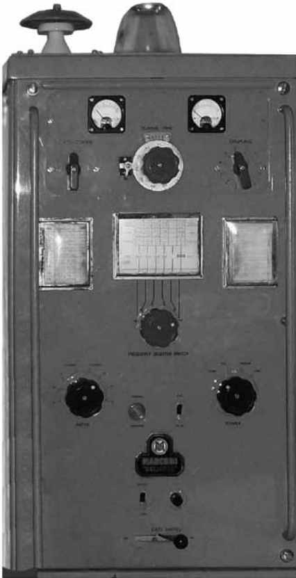
Fig. 10. The Marconi transmitter installed on the on the Reliance was used for classroom instruction. (Jerry Proc collection)
