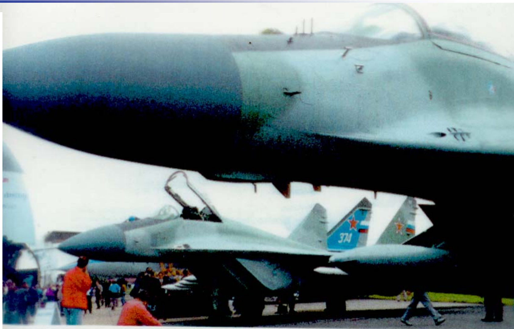
KREMI 2 "EASTERN" IFF ODD RODS TRANSPONDER ANTENNA
