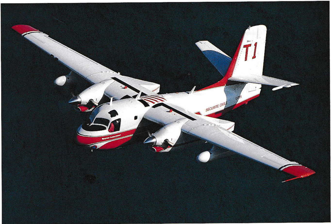
Turbo Firecat 'T1' displays its compact yet purposeful lines during a pre-delivery test flight. The addition of PT6A-67AF turboprops will enable this former RCN Tracker to remain a protector of Mediterranean forests well into the next century. (Keith Wade)
