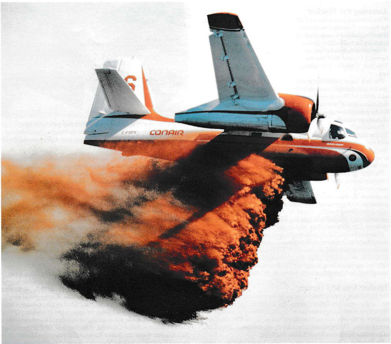
Conair Firecat '566' delivers a load of fire-containing retardant. Full-length tank compartments produce a streamlined charge, reducing erosion during the drop (as indicated by the relatively unbroken leading edge) and resulting in better distribution around a fire. C-FOPV served with the RCN as CS2F-1 1535 and with the Ontario Ministry of Natural Resources as tanker '55'. (via Conair)
