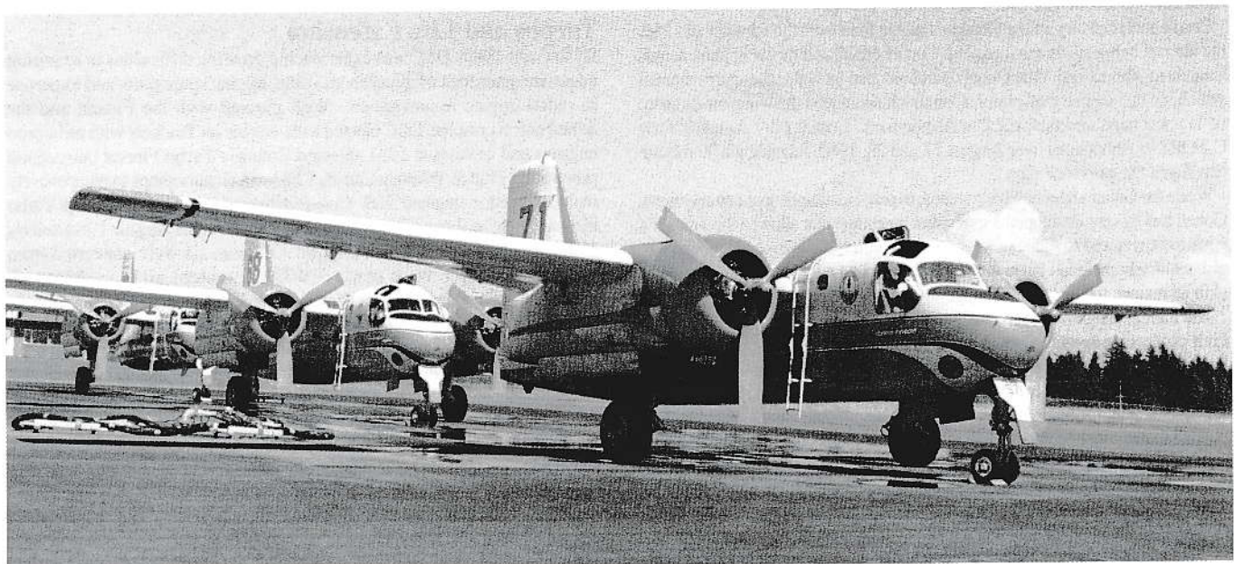
Initial attack group of three Firecats on 'Red Alert' stand-by at the BC Forest Service's Abbotsford Air Tanker Base in July 1995. The first aircraft would be loaded with retardant and airborne within 10 minutes of the dispatch horn sounding. Note the boarding ladder to allow the pilot access to the open port escape hatch. (Author)
