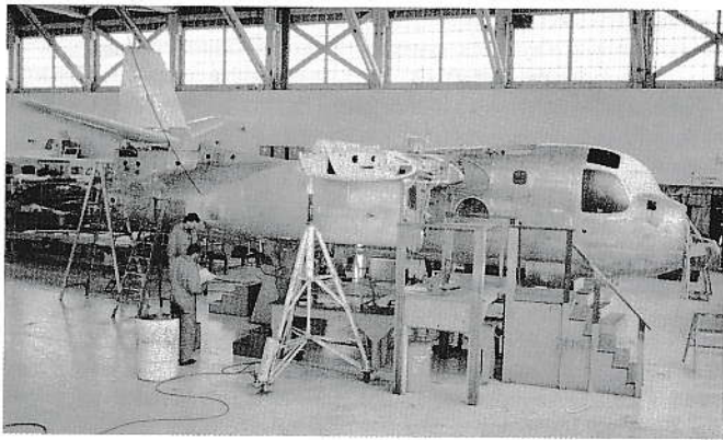
DSC Firecat 'T-1' under conversion to Turbo Firecat configuration in early 1995. Conair completely strips the Tracker airframe and rebuilds all systems to 'as new' condition. (Author)
