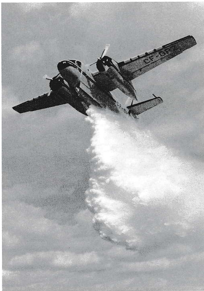
Ontario's proof-of-concept Tracker air tanker CF-OPZ makes a four-door drop of water at Downsview during the 1971 certification trials. Retardant would more normally be delivered in two door salvos or two- or four-door strings. (de Havilland Inc)
