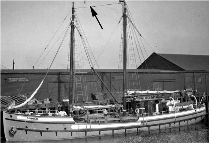
Fig. 9. St. Roch in 1928 showing the cage antenna. (Source: City of Vancouver Archives, public domain, AM54-54 BoN243)
